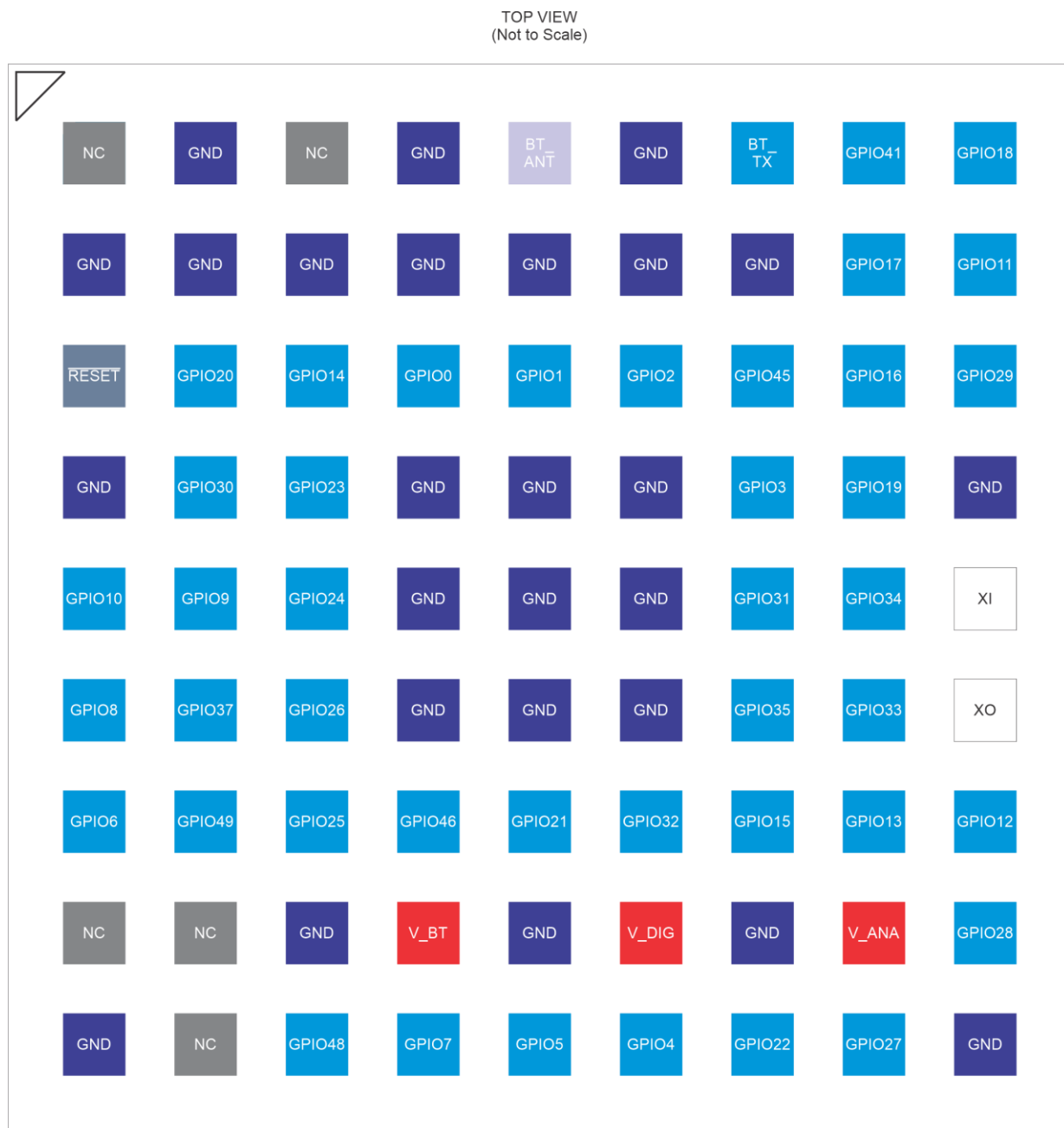
Figure 1: NM180101 Pin Diagram
